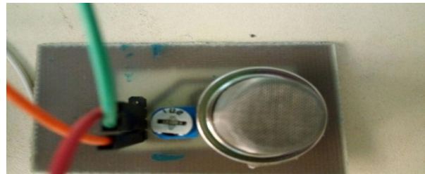
Fig.3.2 MQ135 along with signal conditioning (NH3 sensor)
