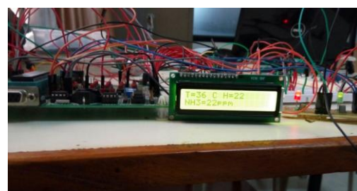
Fig.6 Master controller shows received data using 16x2 LCD based display section
